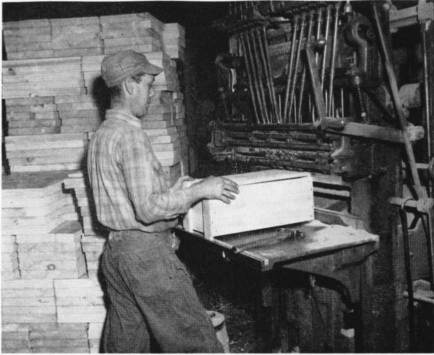
Ernest Boucher, operator of an automatic nailing machine in the Box Shop, is putting on the bottom of a wooden shipping crate. Frank Stanco, another machine operator, performed the first operation on the boxes by nailing the sides together. The two of them can turn out 700 boxes a day.
